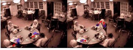
Figure 3. Estimated region motion vectors. The red arrows are computed motion vectors; the blue masks indicate the segmented moving regions.
